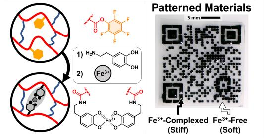
**Figure 1:** (Left) Cartoon overview of polymer network design via active ester chemistry to form networks with mixed iron-catechol and covalent crosslinking. (Right) Demonstration of high resolution patterned materials with specific hard (iron-complexed) and soft (iron-free) domains. The QR code is a link to the publication.
