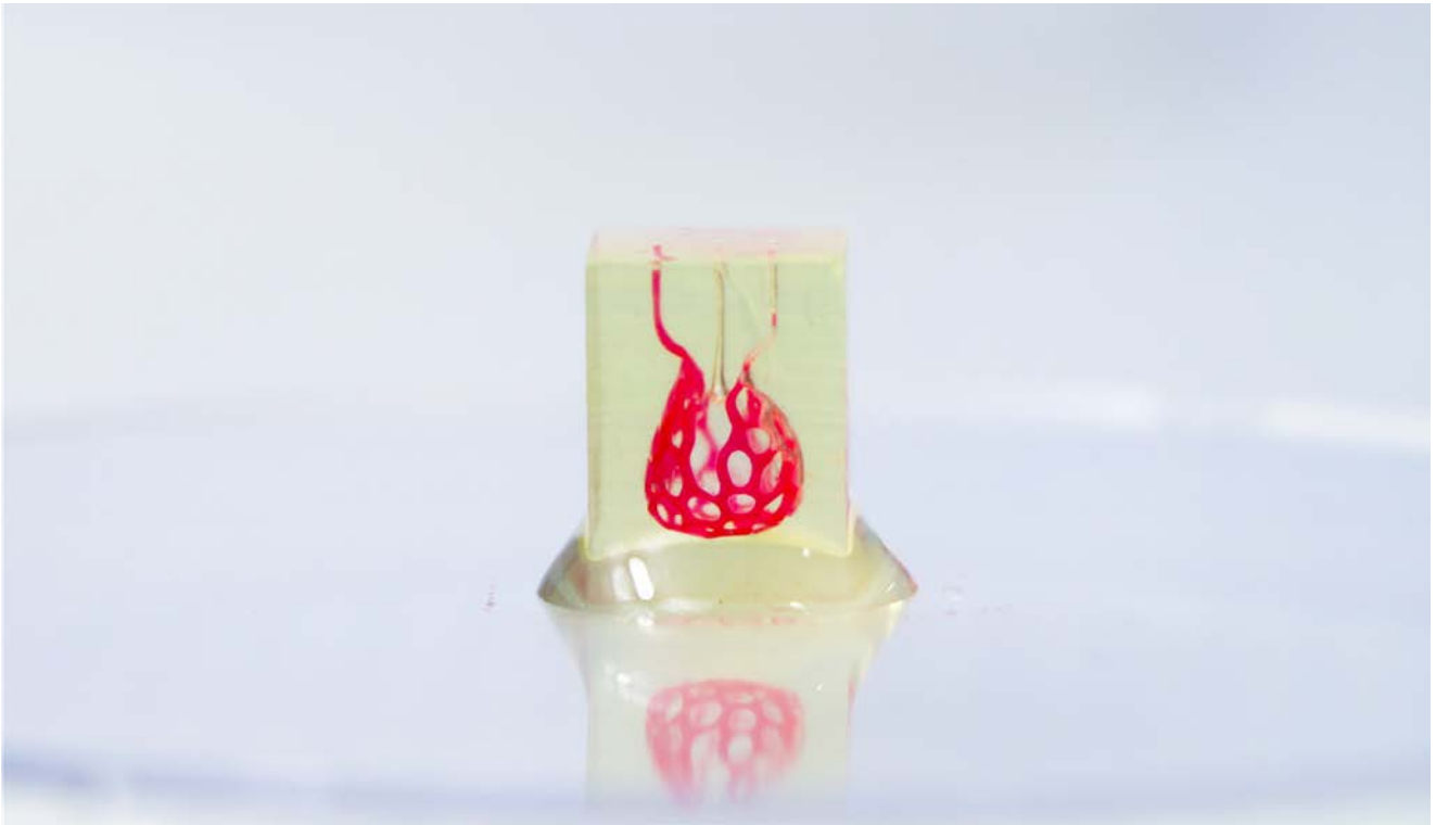
Alveolar cluster (6 x 6 x 9 mm) – Gas exchange network with fluid channels and air inlets. Smallest channel diameter is approximately 250 \mu\text{m} .
